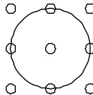
(b) The footprint of a reconstruction filter
